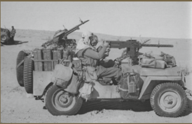
Picture: A heavily armed SAS/LRDG Jeep, armed with a .50inch Browning up front and a Vickers 'K' gun at the rear.
